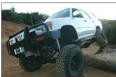
The Pan hard rod relocation bracket drops the pan hard rod by about 2" but with the rear lift at about 5.5" the pan hard rod is still at an angle. The main problem with this is that it causes the rear axle to shift to the right as the rear suspension drops. This causes the drive shaft to hit the gas tank and reduces spring extension because
