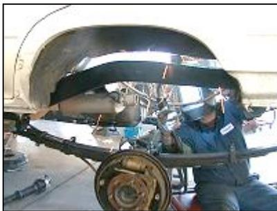
There are a host of other problems associated with modifying the original coil system to accommodate the 5"+ of rear lift I needed to match the front solid axle conversion and clear my 35". When lifting the rear suspension it is necessary to relocate the mounting points so as to level the control arms. If the control arms are not nearly level with the ground the rear axle induces bump steer when the body rolls to one side or you hit a bump with one of the rear tires.
