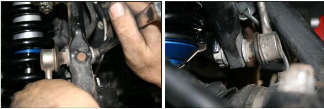
4. Install the longer upper bolt through the heim joint, then the misalignment spacer, then the spindle, and install a flat washer and NyLok nut on the opposite side of the knuckle. \*Blue LocTite Recommended
