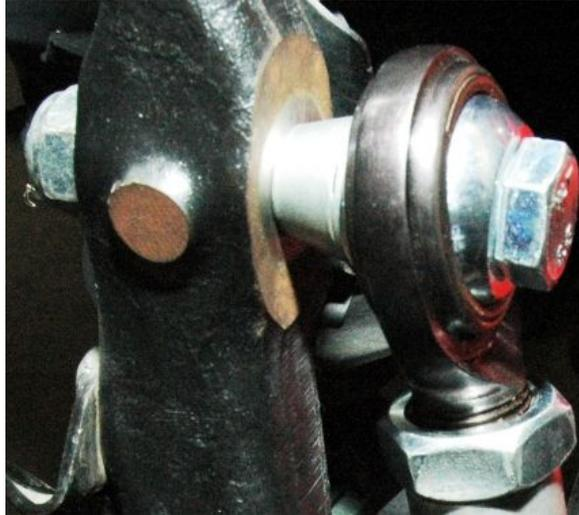
5. Install the shorter bolt through the lower heim, then the spacer & through the sway bar end hole from the outside, and install a flat washer and NyLok on the inside of the sway bar. \*Blue LocTite Recommended
