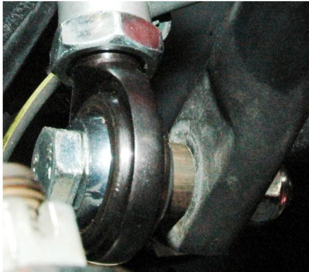
6. Tighten both the nut and bolt with wrenches (approx 60 ft. lbs).
