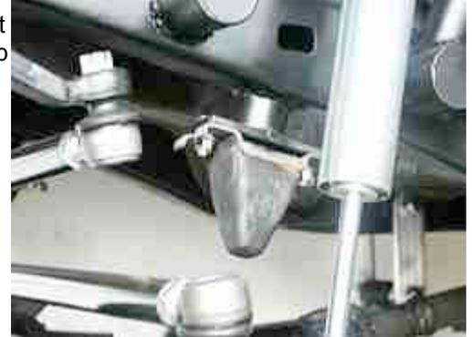
**Shocks** Shocks and shock mounts should be selected that do not limit the travel of the suspension. If it is not possible to install shocks long enough to accomplish this, bumpstops and limit straps should be used to prevent damage to and failure of the shocks.
