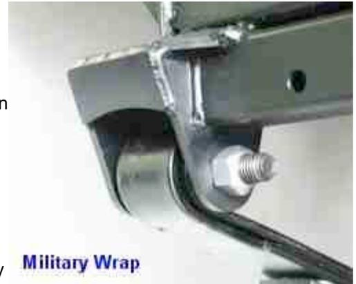
**Military Wrap** Leaf springs should be installed with the military double wrapped end in the fixed spring location. Each leaf spring has a fixed end and a shackle end. Most Toyota pickup's and 4Runners place the fixed mount up front and the shackle in the rear. Thus the military wrap should be in front when mounting springs with the shackle in the rear.
